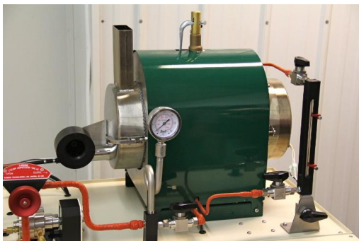
Steam Generation Boiler A dual-pass, flame tube system. If system is cool, open boiler door to reveal boiler construction and flame tube layout. Also note burner fan and tube mounted in door.
